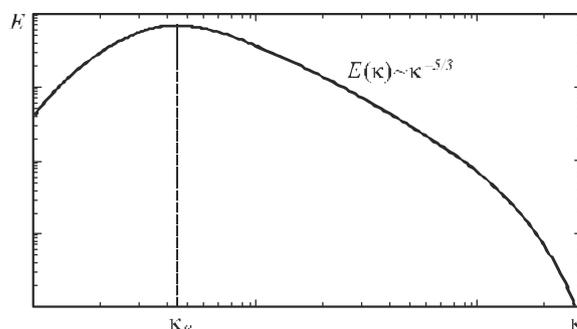
Fig. 1. Energy spectrum in logarithmic scale [33]
