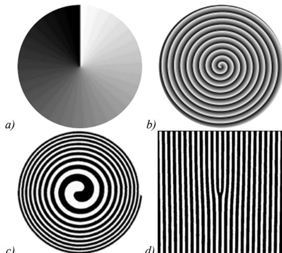
Fig. 7. Elements of singular optics: (a) spiral phase plate, (b) spiral axicon, (c) spiral zone plate, (d) binary “fork”-grating
