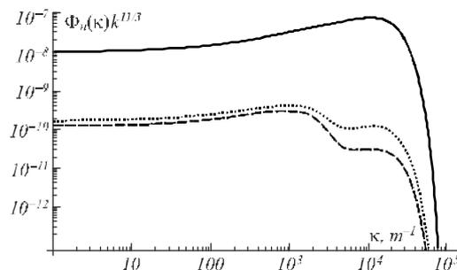
Fig. 5. Oceanic spectrum [84] normalized by Kolmogorov spectrum in the logarithmic scale:  $w_K = -0.1$  solid curve,  $w_K = -2.5$  dotted curve,  $w_K = -4.9$  dashed curve
