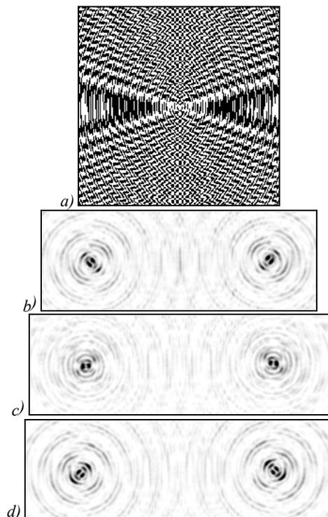
Fig. 9. Experimental generation of rotating laser beams at  $\pm 1$ -st diffractive orders by binary DOE (a) [167]: intensity distributions recorded by CCD-camera at different distances
