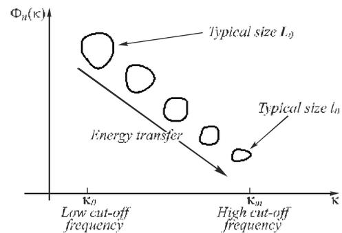
Fig. 2. One-dimensional spatial power spectrum of isotropic turbulence (logarithmic scale)
