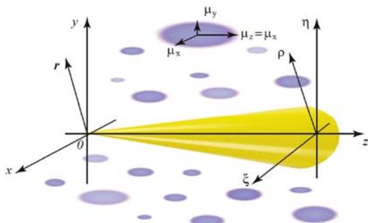
Fig. 4. Anisotropic ellipse of average refractive index fluctuations in atmospheric turbulence
