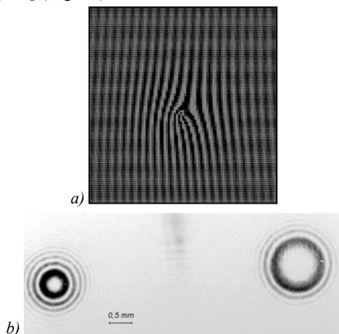
Fig. 11. Experimental generation of vortex hypergeometric beams by coded binary DOE [177]: central part of coded element (a), intensity distributions for convergent and divergent beams with vortex phase of third order (b)
