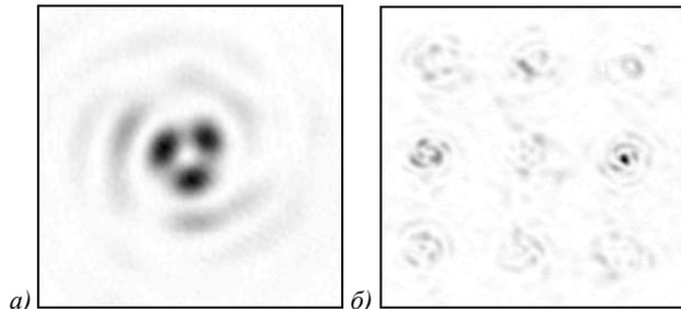
Fig. 13. Experimental detection of optical vortices by means of 8-channel DOE: (a) analyzed beam containing superposition of optical vortices with different orders, (b) focal picture with correlation peaks in accordance with diffractive orders
