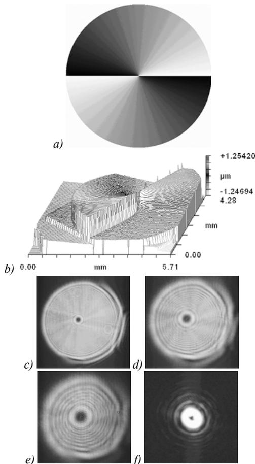
Fig. 8. Experimental generation of laser beam with vortex singular phase of second order [164]: phase distribution (a), central part of spiral phase plate (b) and intensity pictures recorded by CCD-camera at different distances (c)–(e) and at focal plane (f)
