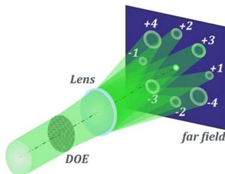
Fig. 12. Action of multi-order DOE with added lens: the coefficients of expansion of the incident field are proportional to the intensity of the corresponding points of the focal plane
