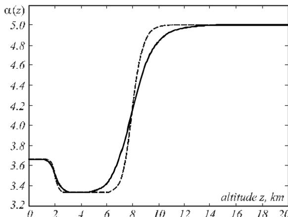
Fig. 3. Three-layer models of non-Kolmogorov turbulence. Two curves correspond to different measurement campaigns [70]
