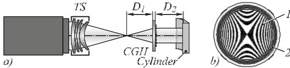
Fig. 2. Optical layout of a Null-Test for cylindrical surfaces using a TS and a CGH (a), main CGH structure '1' and ring CGH '2' for alignment (b)
