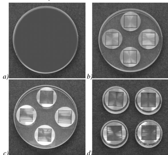
Fig. 4. Main fabrication steps of the CGH: deposition of chromium layer (a), laser writing (b), reactive ion etching (c), separating of the fabricated CGHs by drilling (d)
