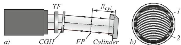
Fig. 1. Schematic diagram of a standard Null-test for cylindrical surfaces using a CGH (a). Main CGH structure '1' and grating pattern '2' for alignment (b)
