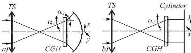
Fig. 3. Optical scheme of the cylinder Null-Test with TS and CGH. XZ-view (a) and YZ-view (b)
