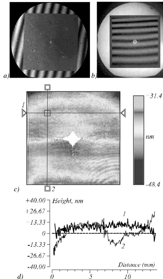
Fig. 6. Interferograms of the alignment hologram (a) and a high precision cylinder surface (b), phase map (c) and cross sections (d)
