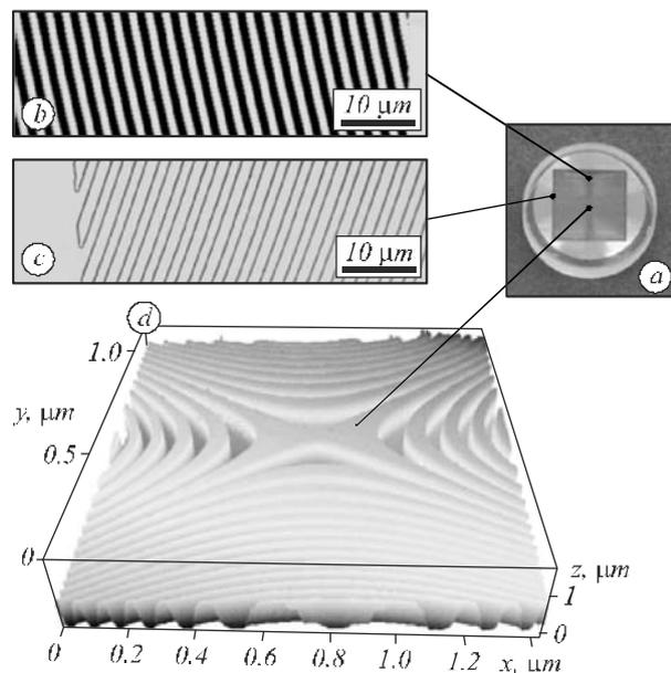
Fig. 5. Fabricated final CGH (a), amplitude pattern of the alignment area (b), phase pattern of the main area at the border (c), 3D representation of the central part of the main CGH (d)
