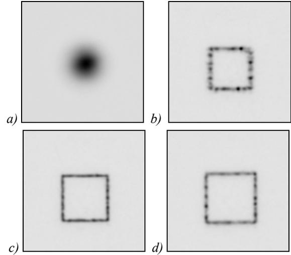
Fig. 9. Experimentally measured intensity distribution in the cross-section of illuminating beam (a) and for different cross sections of the formed beam (“Gauss-to-square contour” focusator): (b)  $z = 90$  mm, (c)  $z = f = 100$  mm, (d)  $z = 110$  mm.
