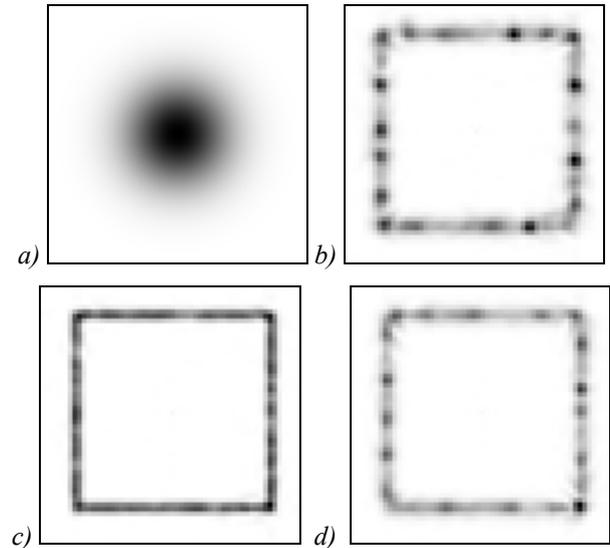
Fig.10. Computer-simulated intensity distribution in the cross-section of illuminating beam (a) and for different cross sections of the focused beam: (b)  $z = 90$  mm, (c)  $z = f = 100$  mm, (d)  $z = 110$  mm.
