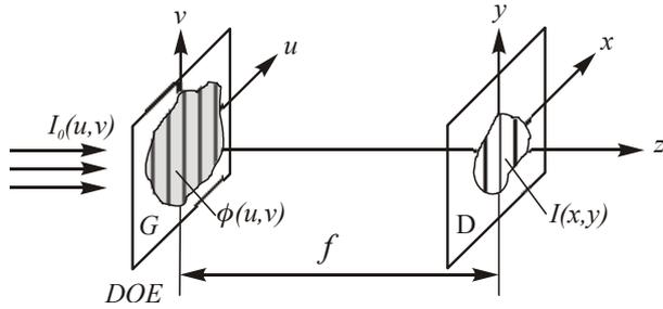
Fig. 1. Principle of laser beam focusing by DOE
