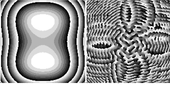
Fig. 2. Phase masks of calculated DOEs: (a) Gauss-to-rectangle focuser, (b) Gauss-to-square contour focuser.
