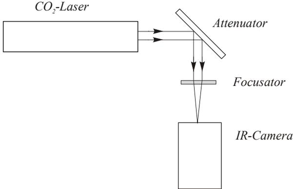
Fig. 7. Experimental setup for the investigation of formed intensity distribution and of diffraction efficiency.
