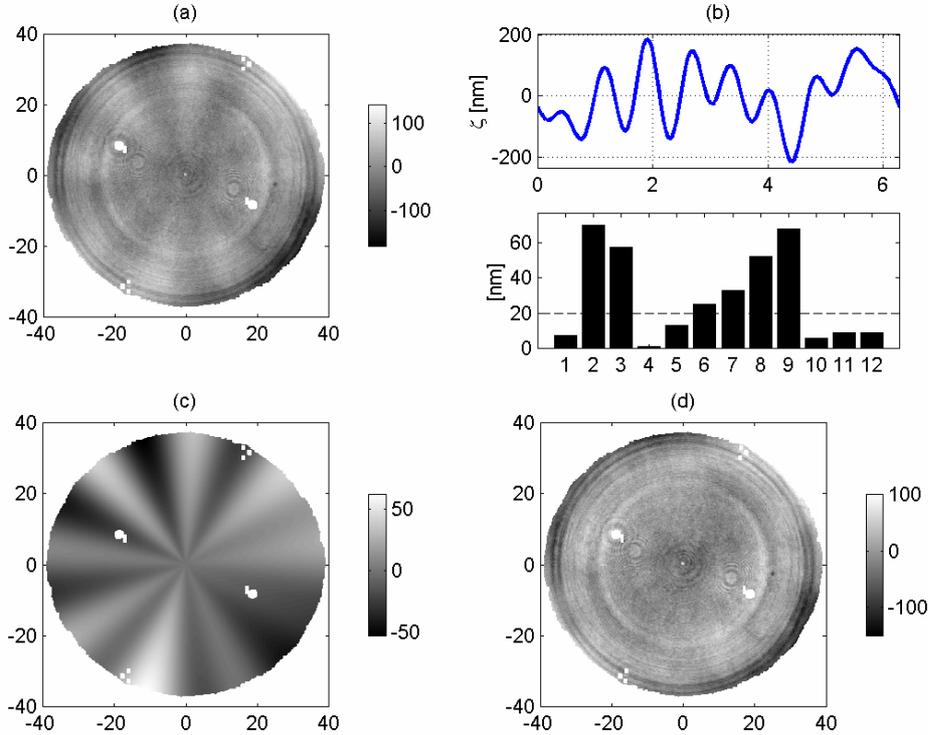
Fig. 6. Numerical elimination of the non-rotationally symmetric wavefront error: (a) Measured wavefront error  $W_{FZL}$ , (b) Frequency analysis of the pattern distortion error  $\zeta_{PD\ NRS}(\theta)$ , (c) Approximation of the non-rotationally symmetric wavefront error, (d) Residual wavefront aberrations after numerical elimination procedure (a) - (c)
