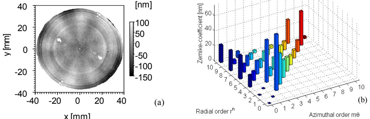
Fig. 5. Residual aberrations of the zone plate  $W_{FZL} = W_{INT} - W_{PLAN}$ . (a) Wavefront error in double pass with  $PV=326$  nm and  $RMS = 38$  nm. (b) Visualization of a 10th order Zernike fit. Main part of aberrations is astigmatism with  $A_{22} = 74$  nm
