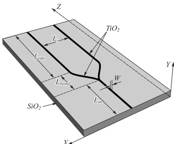
Fig. 4. Schematic of 8 mm long Y-splitter structure with varying distance between two arms ranges from 2–12 μm
