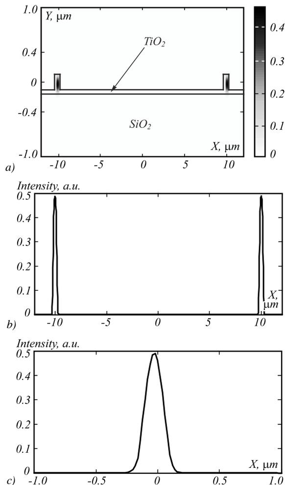
Fig. 6. Simulated results of a Y-splitter at  $0.633 \mu\text{m}$  with a) Mode profile at the output of Y-splitter b) Horizontal cross-section profile of the mode c) Vertical cross-section of the mode
