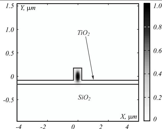
Fig. 3. Simulated single mode of a straight rib channel waveguide
