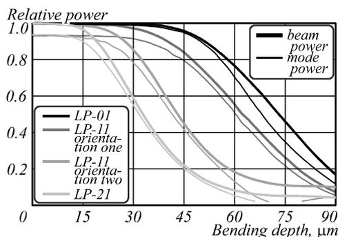
Fig. 9. Beam power in the fiber core depending on microbending depth for LP-01 (the first from the top), two orientations of LP-11 (the second and the third from the top) and LP-21 (the first from the bottom). Thick lines represent full beam powers and thin lines represent mode powers
