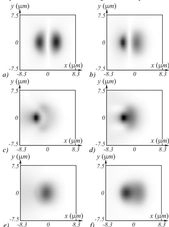
Fig. 8. Amplitude distribution in cross-section (orthogonal to the fiber axis) for the LP-11 mode in orientation two with bending depth of  $74 \mu\text{m}$  for different propagation distances: 0 mm (a), 0.2 mm (b), 0.4 mm (c), 0.6 mm (d), 0.8 mm (e) and 1 mm (f)
