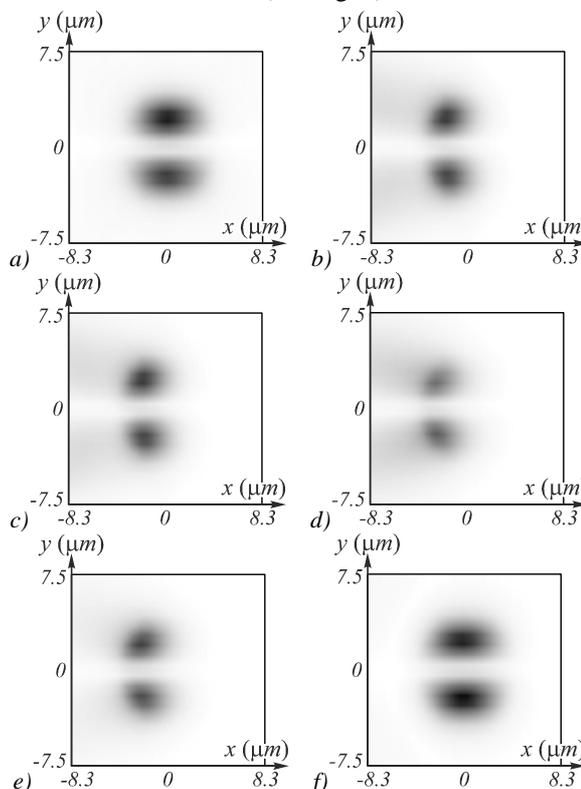
Fig. 7. Amplitude distribution in cross-section (orthogonal to the fiber axis) for the LP-11 mode in orientation one with bending depth of 74 μm for different propagation distances: 0 mm (a), 0.2 mm (b), 0.4 mm (c), 0.6 mm (d), 0.8 mm (e) and 1 mm (f)
