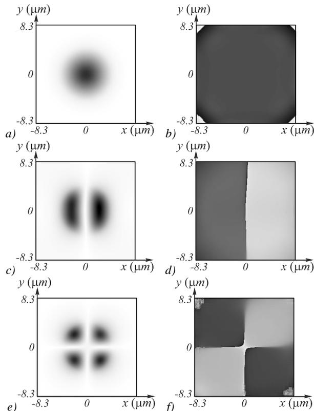
Fig. 2. LP-01, LP-11 and LP-21 modes excitation with Gaussian beam. Cross-section amplitude distributions (a), (c) and (e) and phase distributions (b), (d) and (f) are formed using no microrelief, and microreliefs shown in Fig. 1 (c) and (d), respectively
