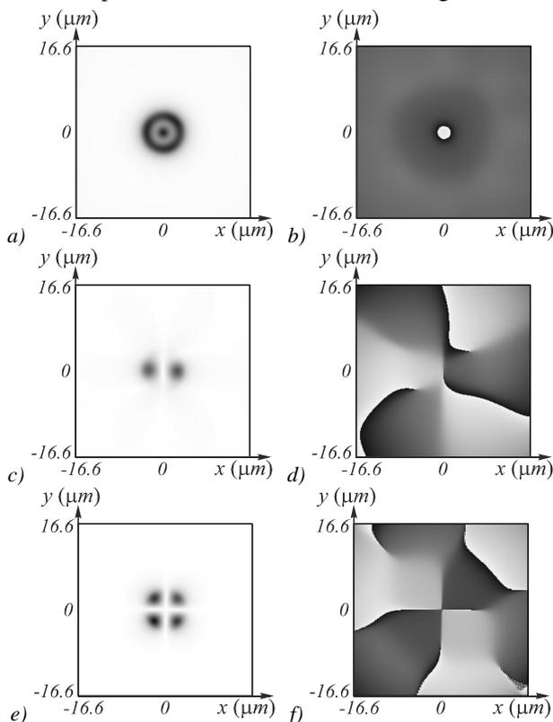
Fig. 4. LP-01, LP-11 and LP-21 modes excitation with Gaussian beam. Cross-section amplitude distributions (a), (c) and (e) and phase distributions (b), (d) and (f) are formed using no microrelief, and microreliefs shown in Fig. 1 (c) and (d), respectively
