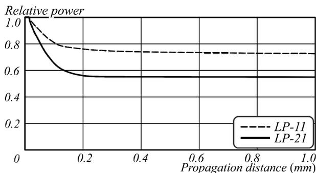
Fig. 3. Beam power in the fiber core depending on propagation distance for LP-11 (upper line) and LP-21 (lower line)
