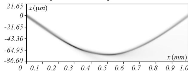
Fig. 6. Amplitude distribution in fiber section for LP-01 mode propagating through fiber microbending (with bending depth of 70 μm)
