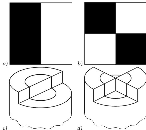
Fig. 1. LP-11 and LP-21 modes excitation. Phase functions (a) and (b) were implemented as microreliefs (c) and (d)
