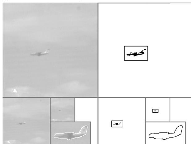
Fig. 2. Image and binary mask at three levels of the pyramid. Black rectangle corresponds to the ROI and is used for contour segmentation
