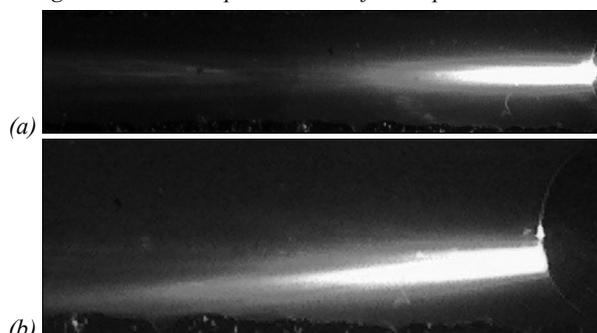
Fig. 2. Photograph of tracks of waveguide modes: (a) left and center of the photo – in the integrated optical NLC waveguide; at the right – planar NLC lens; (b) the focusing effect of a planar NLC lens when the incident beam is shifted to the left of the center. Dimensions on the areas shown in the photo in width are about 3 mm, and in length do not exceed 9–15 mm
