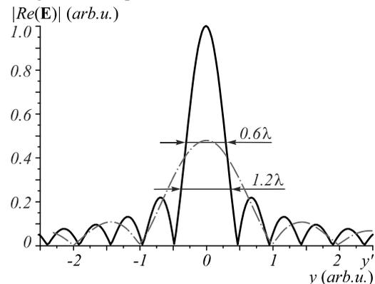
Fig. 6. Distribution of the electric field in the focal plane of the Luneburg waveguide lens presented on the Fig. 7. The solid line corresponds to accounting for 99% of the lens aperture, and the dot-dash line corresponds to 60% of the lens aperture;  $y'=y/\lambda$
