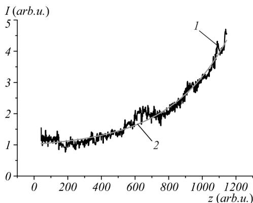
Fig. 3. Dependence of the intensity  $I$  of the scattered laser radiation on the coordinate  $z$  (1 arb.u. $\approx 3.5 \mu\text{m}$ ) with the field  $E$  switched on. TM-polarization. The numbers denote: 1 is the experimental curve, 2 is the fitting exponential curve
