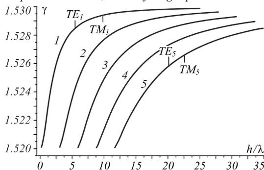
Fig. 4. Dispersion relations for the first five TE and TM modes of NLC waveguide;  $\gamma$  is the effective refractive index of nematic liquid crystal waveguide
