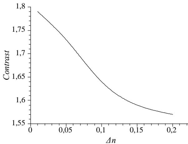
Fig. 8. Dependence of the image contrast  $C$  on anisotropy  $\Delta n$  of the refractive index ( $c = 1.1\%$ ,  $d/\rho_0 = 0.5$ ,  $d = 4\ \mu\text{m}$ )
