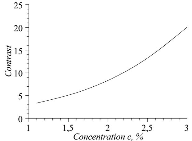
Fig. 2. Dependence of the image contrast  $C$  on the dye concentration  $c$  ( $d = 6 \mu\text{m}$ ,  $\Delta n = 0.2$ ,  $\Phi_T = 900$ )
