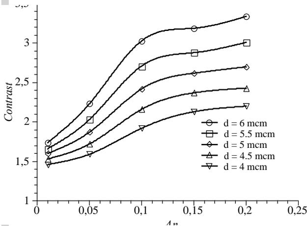
Fig. 1. Dependence of the image contrast  $C$  on anisotropy  $\Delta n$  of the refraction index ( $c = 1.1 \%$ ,  $\Phi_T = 900$ )
