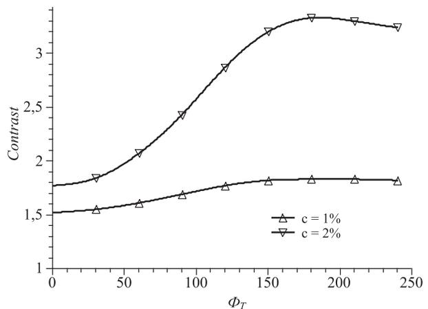
Fig. 5. Dependence of the image contrast  $C$  on the twist angle  $\Phi_T$  of LC structure ( $\Delta n = 0.01$ ,  $d = 6 \mu m$ )
