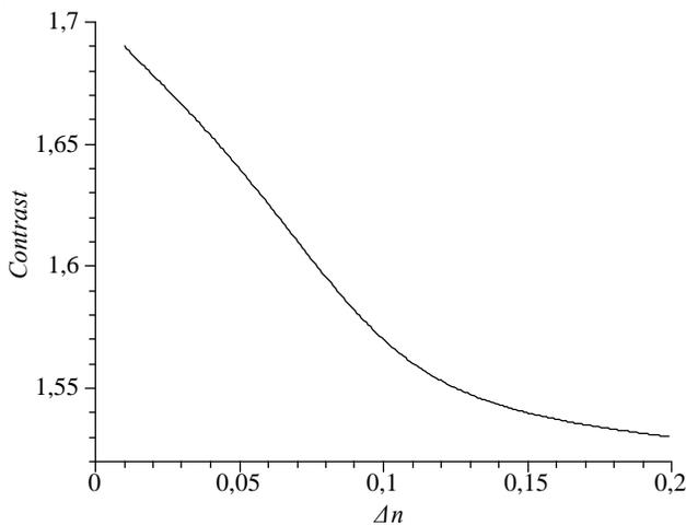
Fig. 4. Dependence of the image contrast  $C$  on anisotropy  $\Delta n$  of the LC transmittance index ( $\Phi_T = 900$ ,  $d = 6 \mu m$ ,  $c = 1.1\%$ )
