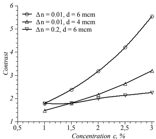
Fig. 7. Dependence of the image contrast  $C$  on the dye concentration  $c$  ( $\Delta n = 0.01, d = 6 \mu m, d/p_0 = 0.5$ )
